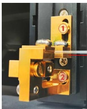
When loosening screws ① and ②, hold this jaw to prevent the filament from damage!
