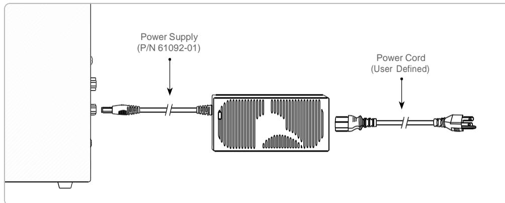
The Microlab 600 uses an external power supply like a computer laptop. The power supply is common to all Microlab 600 instruments and handles 110–220 VAC. When the Microlab 600 is purchased the correct power cord must be selected for the country where the instrument will be used.
