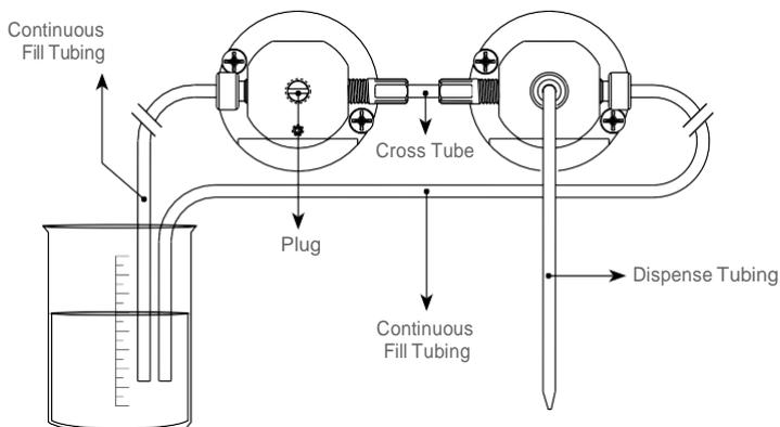
**Note:** All dual syringe pumps will come from the factory set in the diluter configuration. If this is not the desired application, refer to the appropriate configuration and change the pump accordingly.
