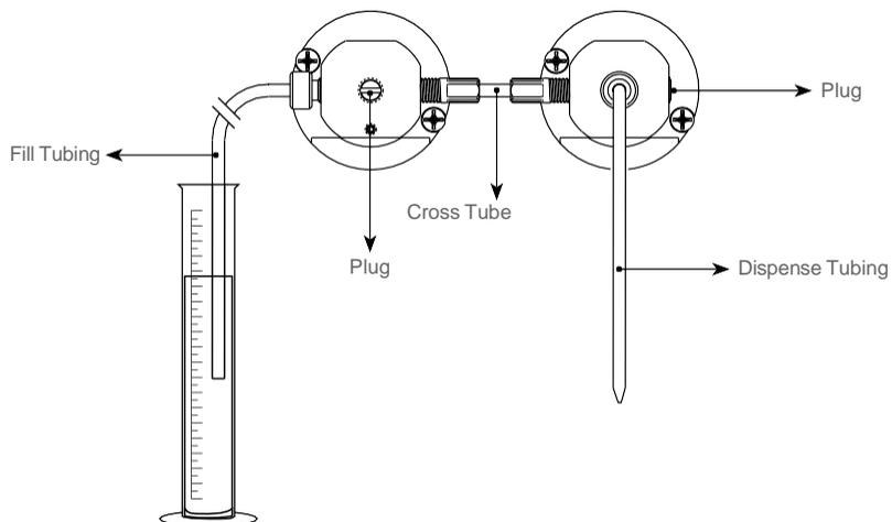
Figure 2-9 Dual Syringe Dispenser Valve and Tubing Assembly
