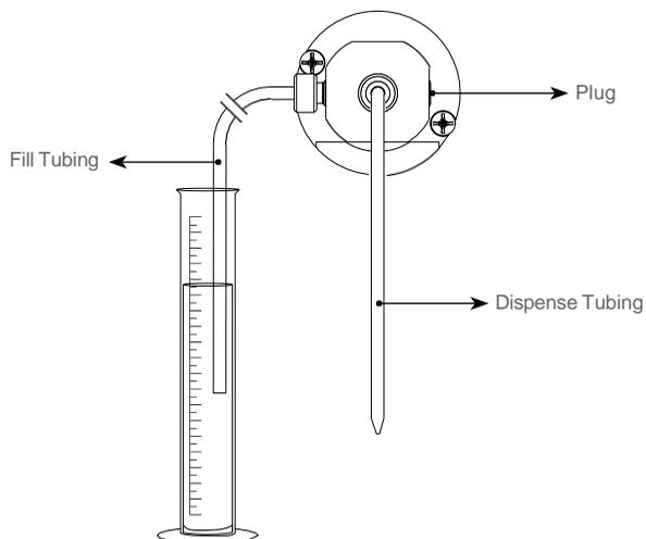
Figure 2-8 Dual Syringe Diluter Valve and Tubing Assembly
