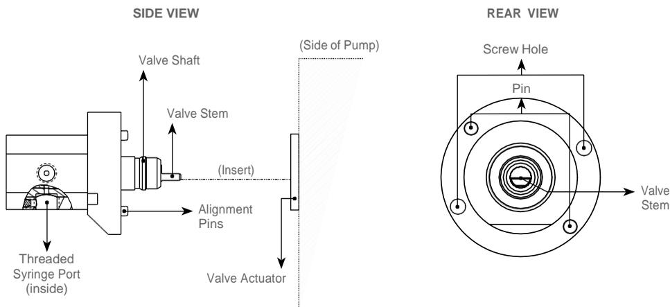
**Note:** The valve assembly will be installed on the Microlab 600 before it leaves Hamilton Company. For single syringe dispensers, the plug configuration will be as depicted in Figure 2-7. For dual syringe units, the valve assembly will be set as a diluter configuration.
