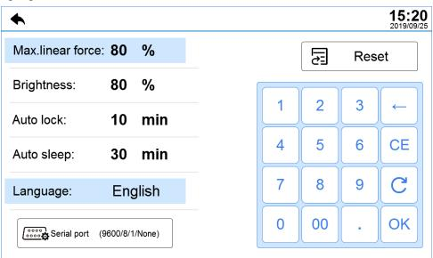
Click [Serial port] to enter the serial port setting interface
