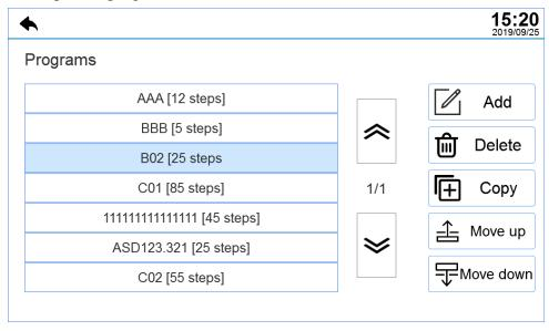
There is a selected program by default in the list, such as "B02 [25 Steps]" in the figure above; click this selected program and enter the program setting interface, as shown in the following figure. Move the position of the selected program via the [Move up] and [Move down] keys in the figure above, or click to select the program and set it.
