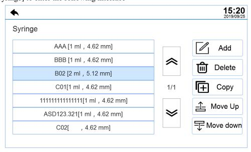
Click [Add] to add a new syringe name, specification and inner diameter parameter, and save them in the syringe management list. The reserved syringe parameter can be called directly when syringe is set.
