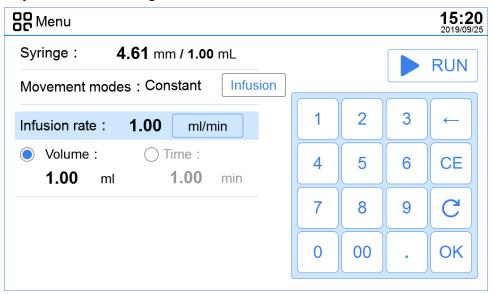
The syringe pump has four movement modes, including: Constant mode, ramp mode, pulse mode and program mode. After system initialization, the equipment enters the [Constant mode] interface by default. Click the [Constant mode] to enter the following interface to switch to the other three modes. Similarly, when in other three modes, click this mode to return to the selection interface and select other modes.
