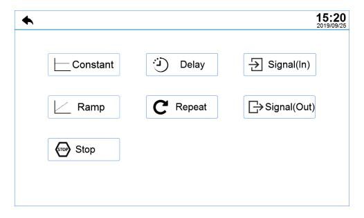
Click [Constant] to set constant steps. For the setting method, please refer to 4.2.1 Description of constant mode setting. Note that the direction of the constant mode here only includes **infusion** and **withdrawal**.
