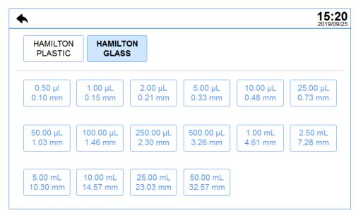
If the syringe used is not included in the default brand, manually set the specifications and inner diameter of the syringe used and then click Save as to save and name the manually set syringe parameters for the future calling. After setting, click [OK] to save the setting, and
